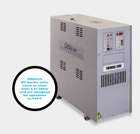
esigned and constructed for many years of dependable operation, the Oiltherm RO Series hot oil temperature controllers come standard with features like automatic oil preheat and fan cooled controls. The multistage centrifugal pump, located in the reservoir, eliminates leaks associated with positive displacement pumps.
